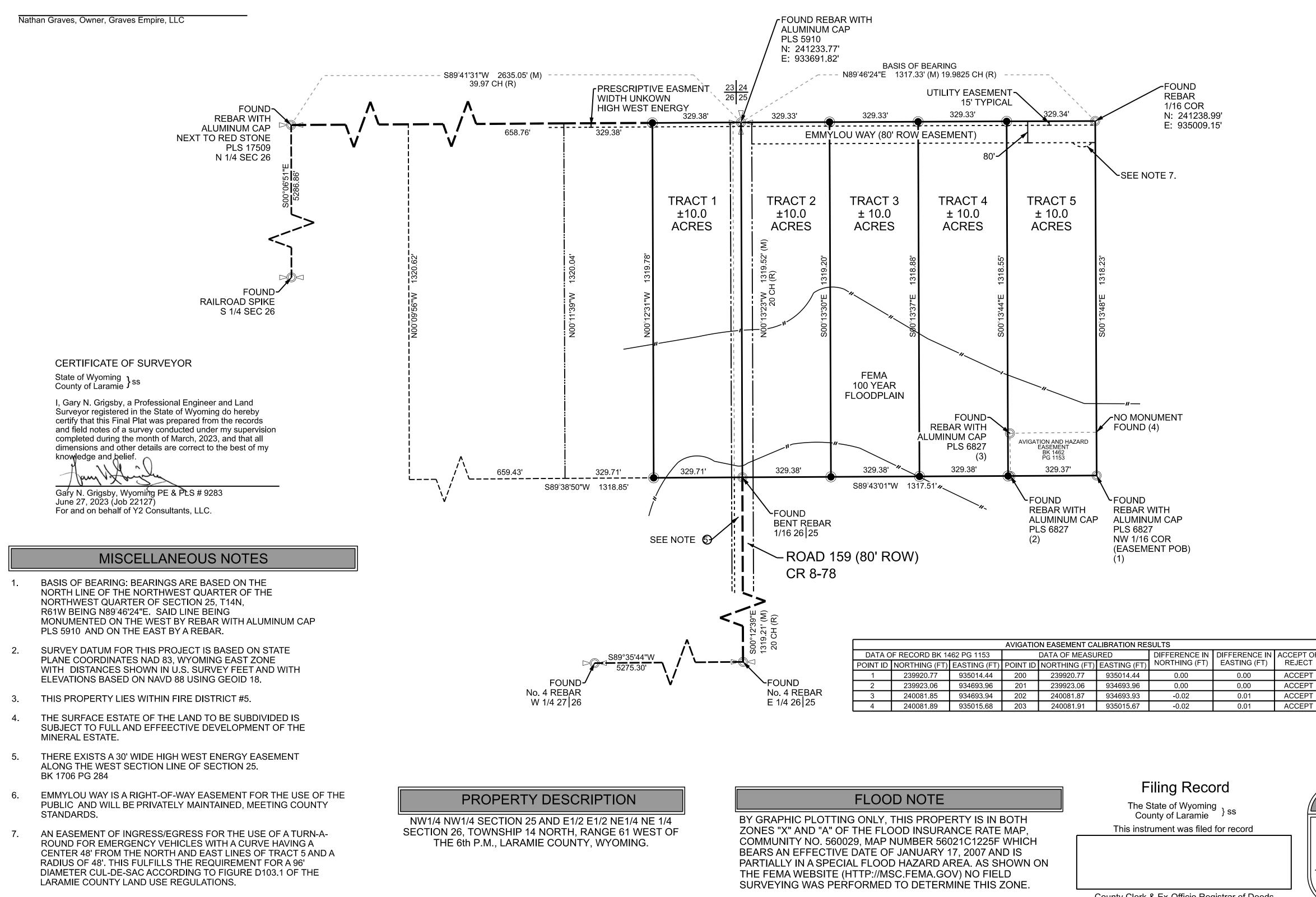
NO CENTRAL WATER SYSTEM OR SEWER SYSTEM ARE PROPOSED FOR THE PROPERTY. THE SURFACE ESTATE OF THE LAND TO BE SUBDIVIDED IS SUBJECT TO FULL AND EFFECTIVE DEVELOPMENT OF THE MINERAL ESTATE. WASTEWATER PERMITS ARE REQUIRED FOR EACH LOT. ALL SMALL WASTEWATER SYSTEMS MUST HAVE A 50' SETBACK FROM ALL PROPERTY LINES AND INTERMITTENT BODIES OF WATER I.E. DRAINAGES AND FLOODPLAINS. A FEMA 100 YEAR FLOODPLAIN RUNS THROUGH SUBDIVISION. SEPTIC SYSTEMS CANNOT BE INSTALLED ON GRADES **GREATER THAN 15%.**
