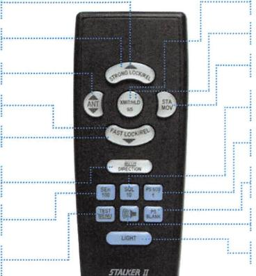
XMIT/HLD – toggles between transmit mode and hold mode.
