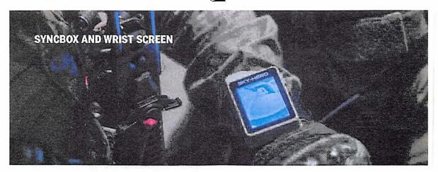
The Syncbox is a portable converter for the stream broadcasted by deployed robots, allowing the transformation of the initial analog signal into a digital format. This digital signal can be injected into any third-party devices with compatible software installed, preferably DroneSense, and ultimately AXON Respond.
