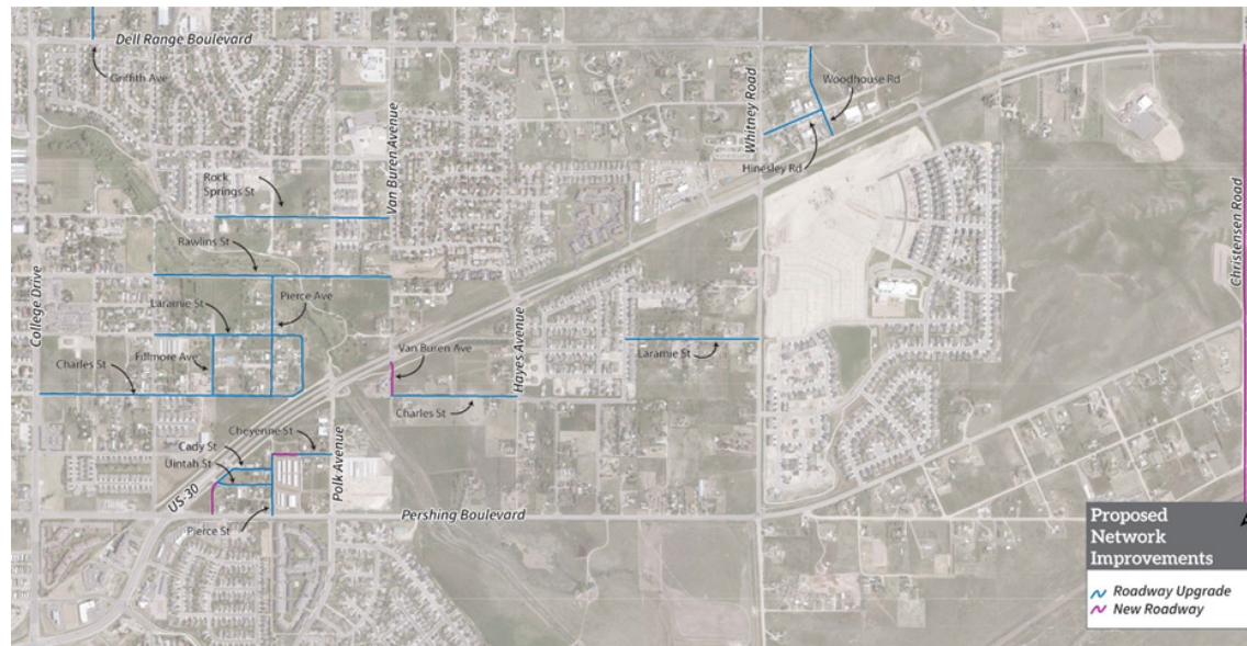
Figure 34: Example Unincorporated Pocket Network Improvements
