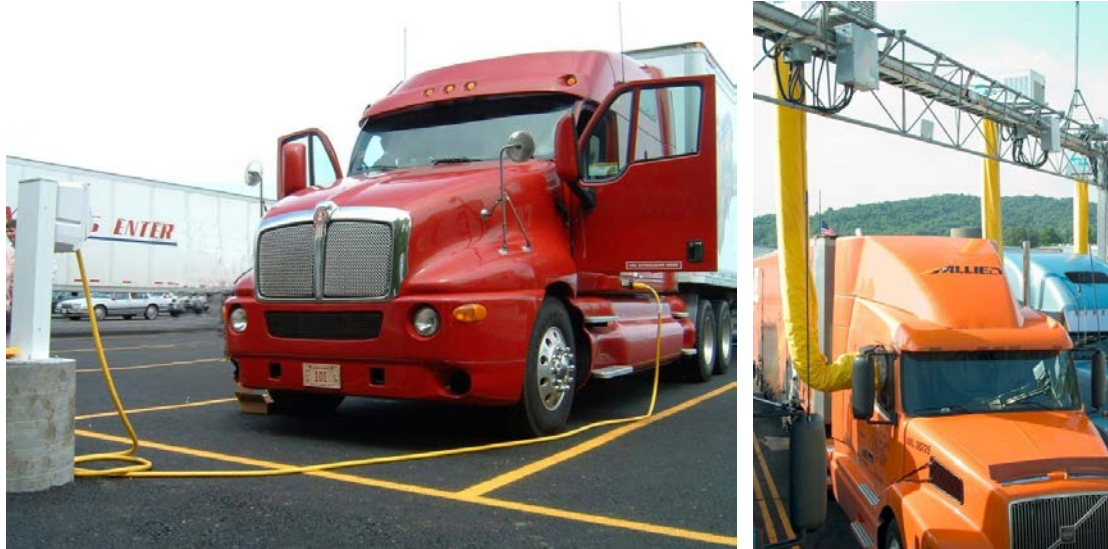
Figure 32: Examples of Truck Stop Electrification
