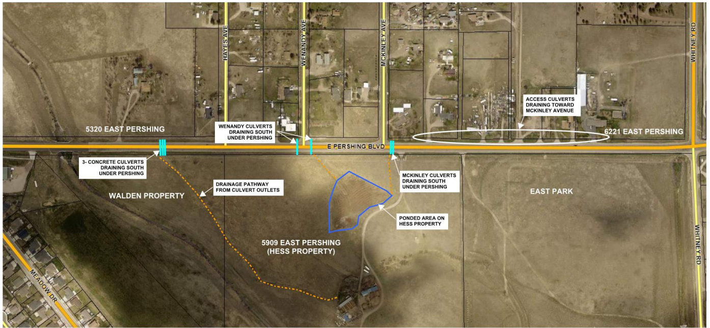
Figure 3: Major Drainage Features from Dry Creek TO 6221 East Pershing Boulevard
