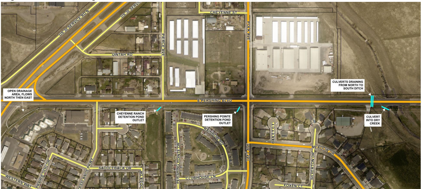
Figure 1: Major Drainage Features from US 30 to Dry Creek
