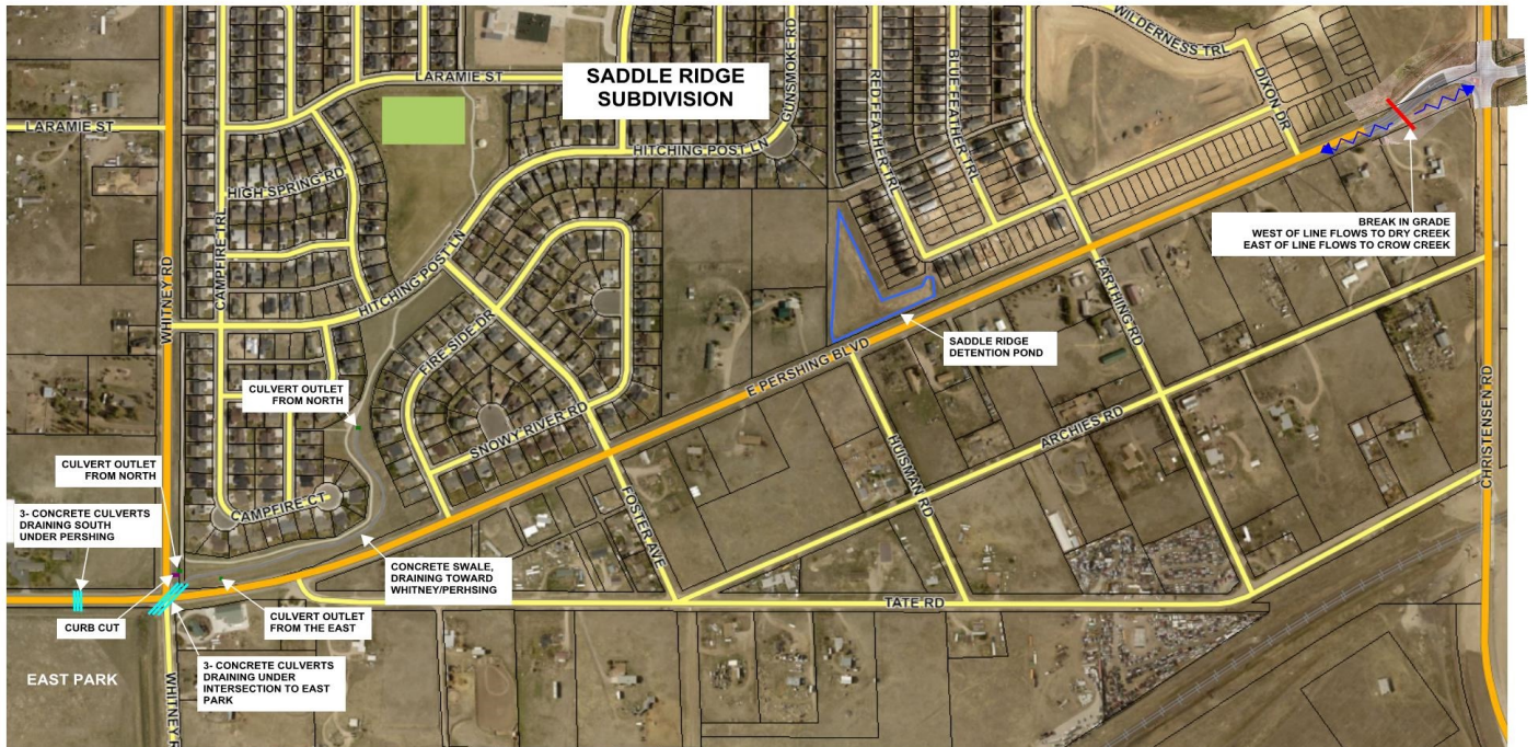
Figure 4: Major Drainage Features from 6221 East Pershing Boulevard to 400 ft west of Christensen Road
