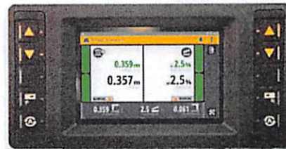
The Trimble Roadworks 2D display features tactile keypads for use in the field
