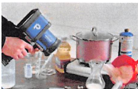
Image 5: High throughput analysis is possible with rapid, touch-free screening.
